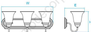
Model No. LV203 Dimension 24"W x 8-1/2"H x 7"E Lamp (3) medium or GU24 base
