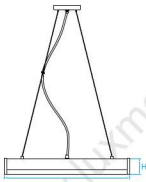
Model No. LP228 Dimension 22"L x 1-3/4"W x 2-3/4"H Lamp 12W integral LED 920 lumens
