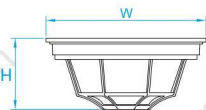
Model No. LO001 Dimension 10-3/4"W x 5"H Lamp (1) medium or GU24 base
