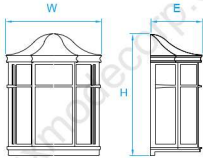
Model No. LO005 Dimension 7-5/8"W x 9-3/4"H x 4-1/8"E Lamp (1) medium or GU24 base 14W integral LED 800 lumens
