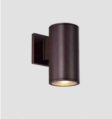
Model No. LO088 Dimension 4-1/2"W x 8"H x 7-1/4"E Lamp 9W integral LED 600 lumens
