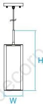
Model No. LP085 Dimension 5-1/8"W x 12-1/4"H Lamp (1) medium or GU24 base
